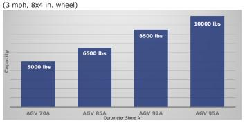
Stellana AGV materials carry high loads at high speed, yet retain the positive attributes of low durometer materials.
