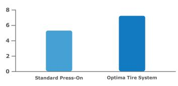
When comparing like tire sizes, The Optima Tire System improves load carrying capacity by over 60% on average or an increase of 2,600 lbs or more.
